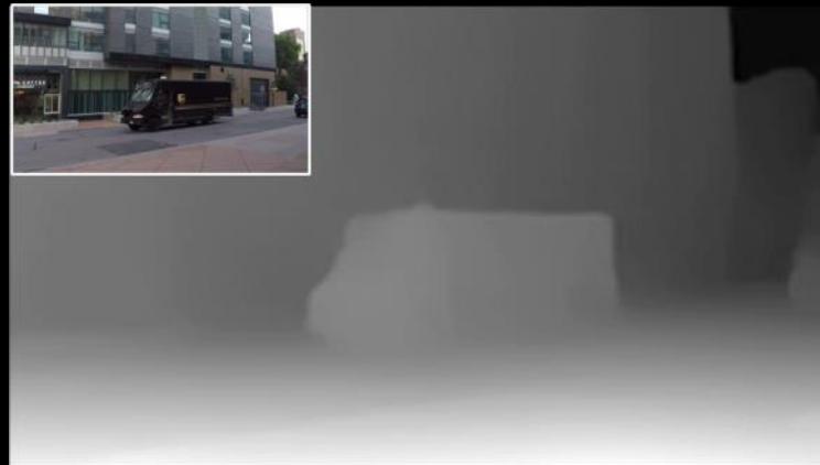
Depth from single-view prediction (scale-variant, complete)
