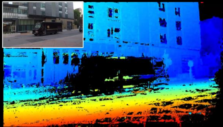
Depth from multi-view stereo (scale-invariant, incomplete)
