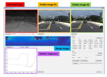
Fig. 6. **Grabber** is a tool for real-time logging and visualization of incoming data from multiple sensors.
